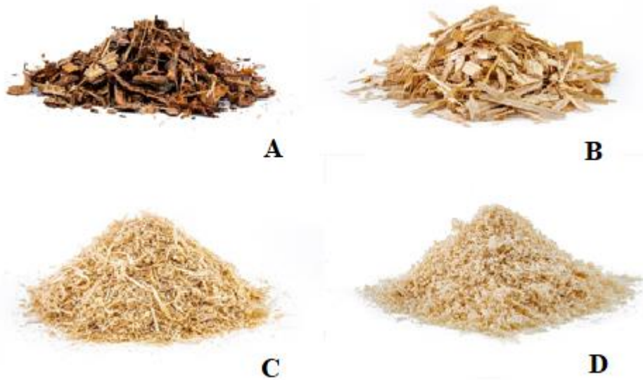
Figure 2. Picture of assortments, A = Bark, B = C-Chips, C = Sawdust and D = Shavings (Persson, L 7 )
