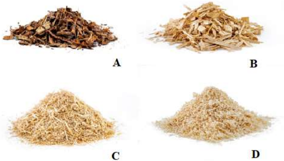
Figure 2. Picture of assortments, A = Bark, B = C-Chips, C = Sawdust and D = Shavings (Persson, L 1 )
